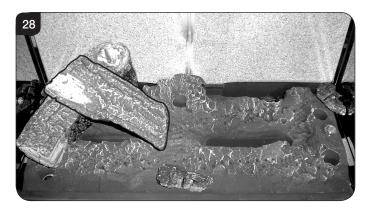
8.21 Place Log C on the right hand side of the burner. There is a hole on the underside of Log C which fits over the raised stud on the right of the burner. The back of the log should rest flush against the back panel, see Diagram 29.
