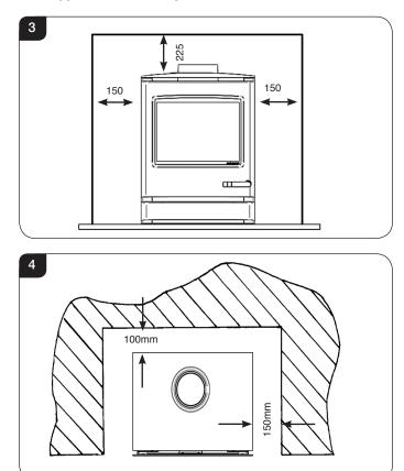
5.10 The above dimensions provide adequate clearance to combustible materials. It may be necessary to add additional clearance so that spillage tests can be performed when necessary.
