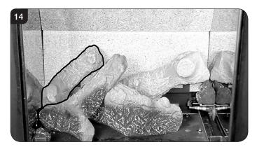
8.7 Place the pointed bottom of log D into the corner of the burner tray and rest on the location stud on log B, see Diagram 15.
