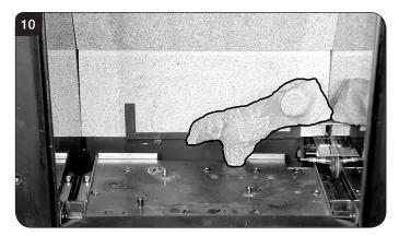
8.3 Place Log B over the two middle studs on the burner tray, see Diagram 11.
