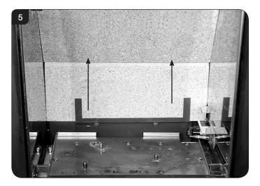
4.5 Slide the lower rear liner up and out of the lower bracket, see Diagram 6.
