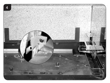
4.4 Gently lift the upper rear liner and pull forwards. With the panel raised it should be possible to remove from the liner brackets, see Diagram 5. Note: It may be necessary to use a flat object like a screwdriver to separate the two panels.
