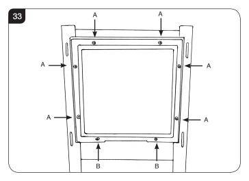
9.2 Replace ALL of the glass frame securing screws ensuring that a screw is present in all fixing slots.
