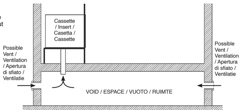
**GB:** Terminations should be made with a proprietary fixed open external air vent kit, which gives minimum free area of greater than listed, positioned so no blockage can occur and not permit the entry of birds or animals.
