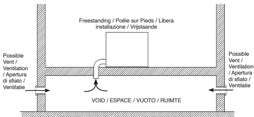
**INTERNAL POSITIONING OF THE AIR DUCT / FIXATION DU KIT SUR L'APPAREIL - INSERT /**
