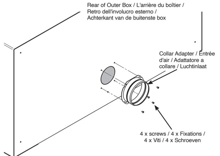
**GB:** Thread the Fixing Band onto the air duct and attach to the Collar Adapter. Secure in position by tightening the integral screw.
