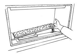
Slide the burner to the right and out of its location.
