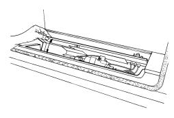
Disconnect the two cables marked 'A'.
