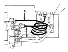
Remove the pipe and the injector drops out from the burner.
