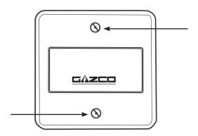
Unclip the battery holder from the wall plate and remove the old batteries.
