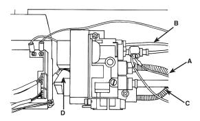
Remove the thermocouple from the interrupter block and release the second thermocurrent cables.
