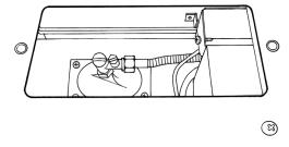
Remove the six screws securing the control assembly.
