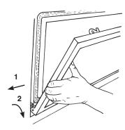
Slide the frame to the right so it comes off the right hinge pin. The window frame should now be free.
