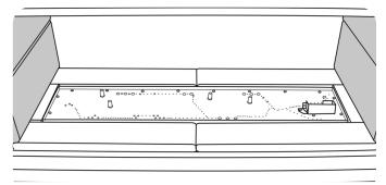
Remove the lower liners around the burner tray.
