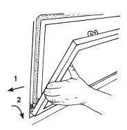
Slide the frame to the right so it comes off the right hinge pin. The window frame should now be free.
