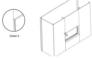
Apply a plaster finish to the chimney breast using heat resistant plaster in the area directly above the appliance.
