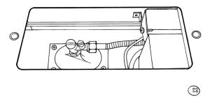
To leak test any gas joints on the appliance the control assembly must be undone and tilted backwards, see page 36, Main Control Assembly.
