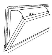
Remove the securing spring clip from the bottom-right of the window frame.
