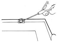
Lift the glass clear from the lock bracket at the top of the frame and slide out.
