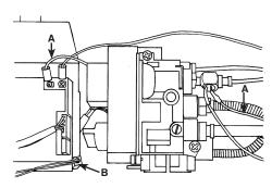
Disconnect the battery extension lead, B.
