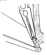
With the window frame in an upright position slide the frame to the left so that it comes off the left hinge pin (1).
