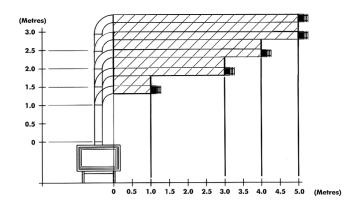
Start of bend to centre line of horizontal flue 170mm. Centre line of vertical flue to end of bend 220mm.
