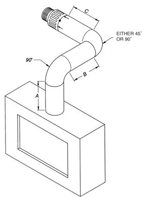
When A = 1.0 to 1.490 metres No additional bend allowed When A = 1.5 to 1.990 metres B + C = 2.0 metres maximum When A = 2.0 metres to 2.490 metres B + C = 4.0 metres maximum
