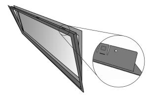
If the Edge+ is too loose the tabs can be bent up to gain better purchase on the edge of the appliance box.
