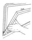
Manoeuvre the frame up towards the left side to locate the left hinge pin.
