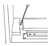
Slide the burner fully to the left and lift the right side clear of the pilot.
