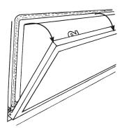
Remove the securing spring clip from the bottom-right of the window frame.
