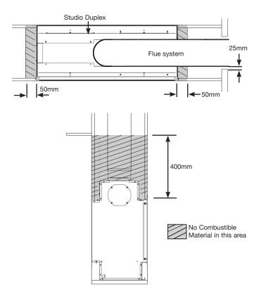
DO NOT PACK THE VOID AROUND OR ABOVE THE APPLIANCE WITH INSULATION MATERIALS SUCH AS MINERAL WOOL.
