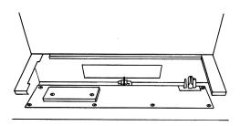
Isolate the gas supply at the isolation device and disconnect the gas inlet.
