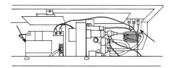
Remove the ignition lead from the electrode, removing cable ties where necessary.
