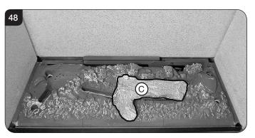
12.5 Place the front of Log J on the raised stud on Log C. The back of the log rests on the rear bracket and touches the pilot bracket, see Diagram 49.
