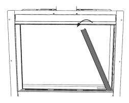
Lift out the bottom slotted trim. Note the orientation of the battery box for reassembly.
