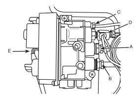
Remove the 2 screws securing the valve to the support bracket and withdraw the valve.
