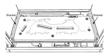
Remove the 4 screws from the corners of the burner unit.
