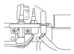
When replacing the pilot ensure the thermocouple follows its original route, i.e. along the pilot pipe. Attach the thermocouple to the pipe with new cable ties.
