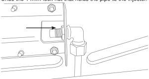
Replace with the correct size injector.
