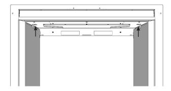
To remove the Right Hand liner first tilt inwards towards the centre of the firebox before lifting up and pulling out through the front of the firebox.
