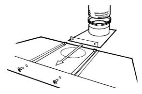
Place the liner in its final position ensuring that the sliding flue plate rests at the correct height in the opening, and that the front flange of the plate rests against the outside face at the top of the opening.
