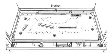
Replace the 4 screws in each corner of the burner unit.
