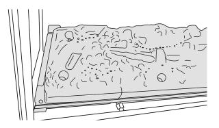
Slide the left hand side forward ensuring the burner tray and splitter plate fits around the mounting bracket.
