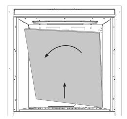
When replace the rear liner, ensure that the 2 brackets are replaced.
