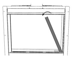
Lift out the bottom slotted trim. Note the orientation of the metal shield for reassembly.
