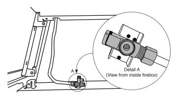
**PURGE THE SUPPLY PIPE**. This is essential to expel any debris that may block the gas controls.
