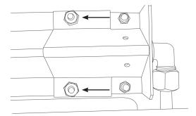
Undo the 14mm lock nut that holds the pipe to the injector.
