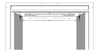
Replace the baffle ensuring that the 3 tabs fit into the slots at the back of the appliance. Take care not to damage the liners.
