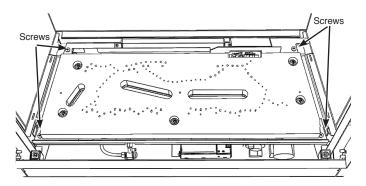
Fit the 2 side brackets supplied in the appliance fixing kit.
