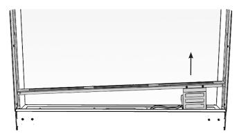
Disconnect the battery lead from the battery pack attached to the lower slotted trim.
