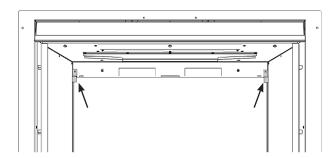
Remove the back liner by carefully lifting over the bottom bracket and twisting slightly to allow it to be removed through the front of the appliance.
