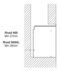
This appliance is not suitable for installation onto a combustible wall; all combustible materials must be removed from the area shown.
