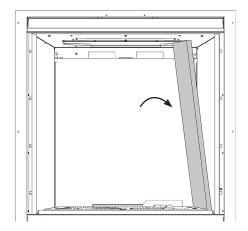
To fit the Left Hand liner insert through the front of the appliance tilting the top inwards towards the centre of the firebox before lowering into position.
