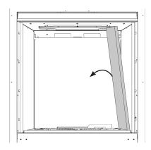
To remove the Left Hand liner first tilt inwards towards the centre of the firebox before lifting up and pulling out through the front of the firebox.
