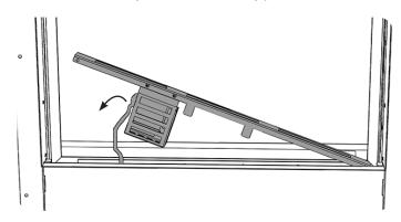
Remove the battery pack from the bracket.
