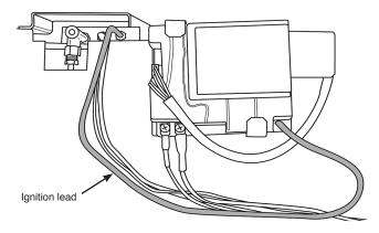
Replace with a new ignition lead following the original route. Refit the Vidaflex cover over the lead. Ensure the cover engages fully over the electrode.
