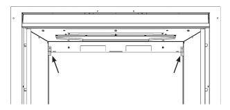
To fit the Right Hand liner insert through the front of the appliance tilting the top inwards towards the centre of the firebox before lowering into position.
