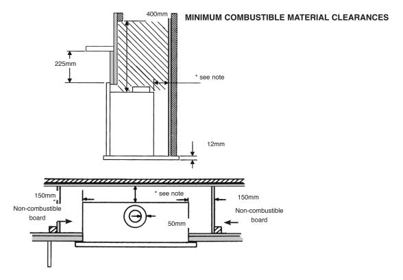
\* All combustible materials must be removed from behind the appliance or a minimum distance of 100mm is required where the combustible material is protected by non combustible board.
