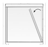
Lift out the bottom slotted trim. Note the orientation of the battery box for reassembly.
