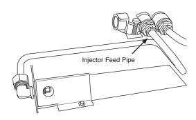
Remove the Aeration plate by unscrewing the two nuts that hold the plate in place.
