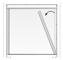
Lift out the bottom slotted trim. Note the orientation of the battery box for reassembly.
