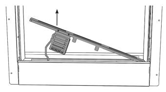
Disconnect the battery lead from the battery pack attached to the lower slotted trim.
