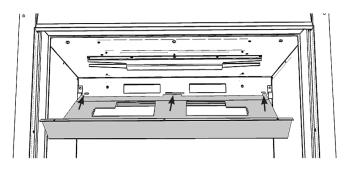
Replace the screws (x2 600/ x3 600HL) to secure it to the roof of the firebox.
