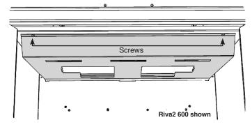
The baffle can now be removed by lowering the front edge and pulling forward through the front of the appliance.
