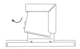
Remove the cover by sliding off in the direction of the arrow as shown.
