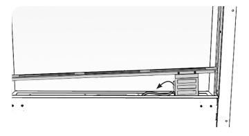
Remove the screws at the base of the glass frame.
