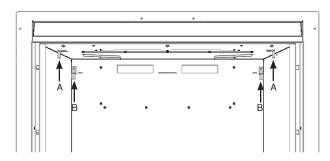
Fit the back liner by carefully twisting slightly to insert through the front of the appliance and lifting over the rear bracket.
