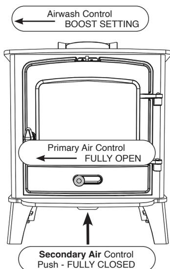
The door must always be closed when operating and must only be opened for adding fuel, ignition and deashing.
