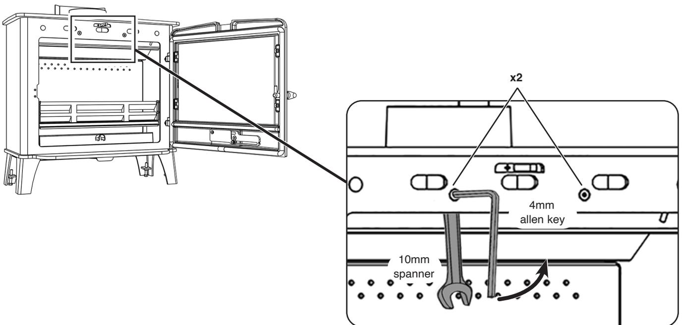
Loosen the hex bolt until the slider moves with no resistance. Once happy with the sliding action tighten the 2 locknuts.
