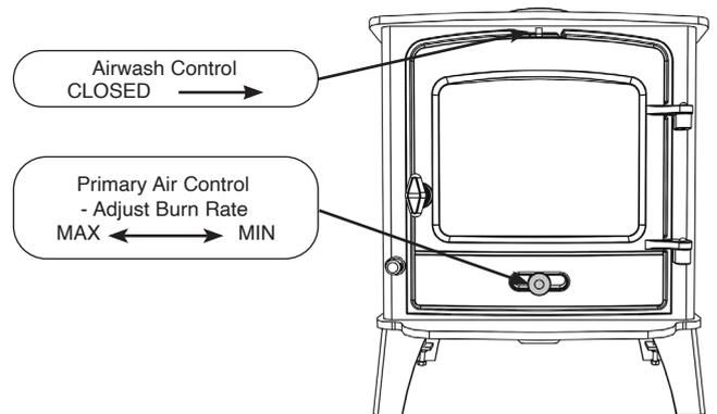
To burn solid fuel efficiently it is best to control the burn rate using the **Primary air control** only.
