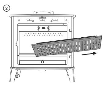
The Door Tool can be used to remove the Ash Pan.
