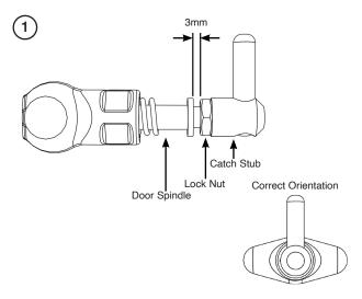
Screw the catch stub up to the lock nut. Ensure the correct orientation of the pin and knob.
