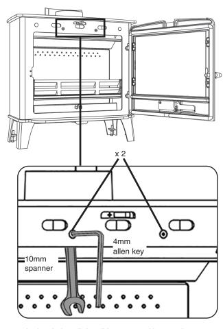
Loosen the hex bolt until the slider moves with no resistance. Once happy with the sliding action tighten the 2 locknuts.
