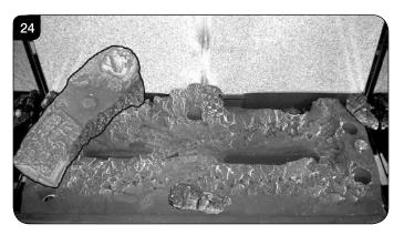
8.20 Place Log B on top of Log D. There is a hole on the underside of Log B which fits over the raised stud on Log D to secure in place. The right hand side of the log rests in the groove in the burner, see Diagram 25.
