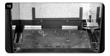
7.2 Place Log A on the higher rear bracket and push up against the back panel, see Diagram 16.
