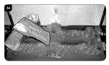
7.21 Place Log C on the right hand side of the burner. There is a hole on the underside of Log C which fits over the raised stud on the right of the burner. The back of the log should rest flush against the back panel, see Diagram 35.
