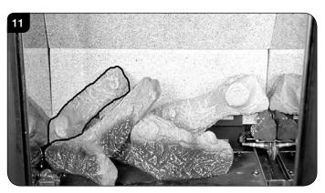
8.7 Place the pointed bottom of log D into the corner of the burner tray and rest on the location stud on log B, see Diagram 12.
