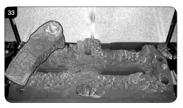
7.20 Place Log B on top of Log D. There is a hole on the underside of Log B which fits over the raised stud on Log D to secure in place. The right hand side of the log rests in the groove in the burner, see Diagram 34.
