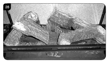
8.24 Sparingly spread an amount of the Embaglow fibres provided and ensure the ports in the burner tray are covered, see Diagram 29. Take care not to use more than half a packet per application.
