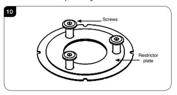
Remove the restrictor plate that is current in place and fit the  $40\text{mm}\ \varnothing$  one from the kit.
