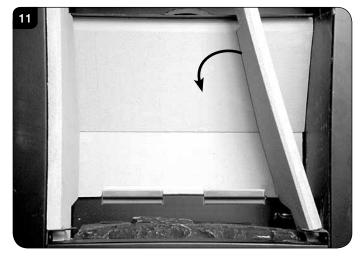
4.10 To remove the Right Hand liner first tilt inwards towards the centre of the firebox before lifting up and pulling out through the front of the firebox, see Diagram 11.
