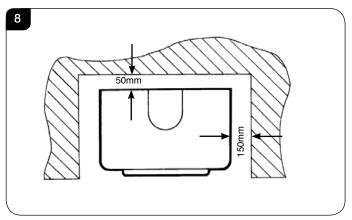
7.4 In a non-combustible recess be careful to allow enough clearance at the sides and rear of the appliance to perform spillage tests and reach the controls.
