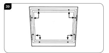
8.3 Replace ALL of the securing screws ensuring that a screw is present in all fixing slots.
