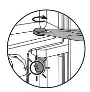
To release the pin, retract the barb using flat pliers and pull the pin upwards.
