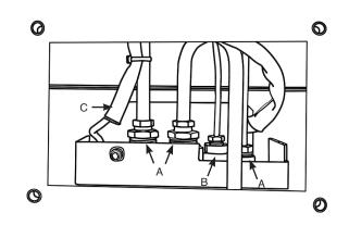
Disconnect the ignition lead from the gas valve, (C).
