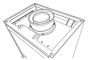
Remove the 8 screws securing the inner & outer spigots.
