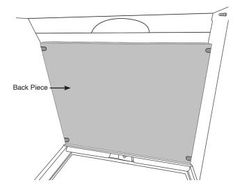
With the liners and baffle removed the firebox is clear for cleaning and maintenance.
