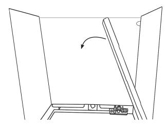
Support the rear panel when handling the last side and remove carefully.
