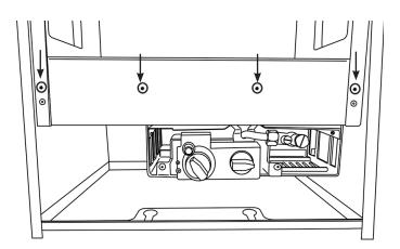
The frame can be removed by lifting the hooks clear of the slots from the bottom of the frame and lifting away from the appliance.
