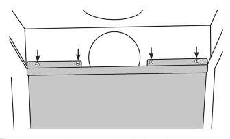
To make removal of the rear panel easier, it may be necessary to remove the burner tray.
