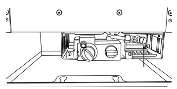
Connect a suitable pressure gauge to the test point located on the inlet fitting and turn the gas supply on. Light the appliance and check all gas joints for possible leaks. Turn the appliance to maximum and check that the supply pressure is as stated on the databadge. Turn the gas off and replace the test point screw, turn the gas on and check the test point for leaks.
