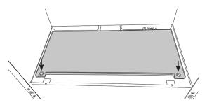
Lift the burner out of the firebox at an angle clear the brackets, exposing the service hatch.
