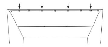
The baffle can now be removed through the front of the appliance.
