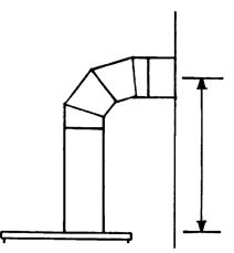
TAKE CARE TO MARK OUT THE FLUE CORRECTLY. IT IS DIFFICULT TO MOVE AFTER INSTALLATION.
