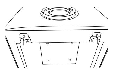
Attach the supplied Gas pipe extension to the gas inlet of the appliance.
