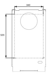
Position the wall mounting bracket in the required location.
