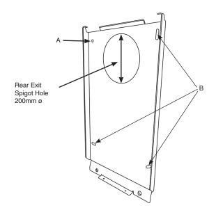
Level the wall mounting bracket and mark the remaining 3 holes, arrow B.
