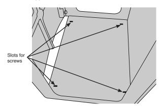
Remove the appliance and drill the guide holes.
