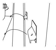
Take care when fitting the back panel not to catch the gas inlet extension pipe. This will protrude from the cutout at the bottom of the panel.
