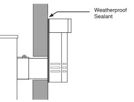
Feed the flue through the wall, making sure it runs smoothly.
