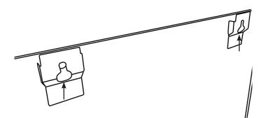
Lower the panel and hook the lower brackets over the edge of the appliance body mid way down.
