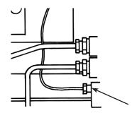
Reassemble the interrupter block and leads and secure the thermocouple connection in the rear of the gas control. (Do not overtighten).
