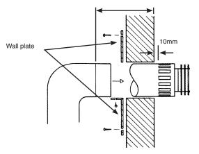
Mark the correct length all the way around the flue terminal section.
