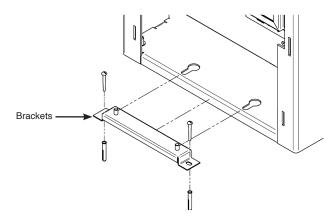
Remove the bracket and drill the guide holes.
