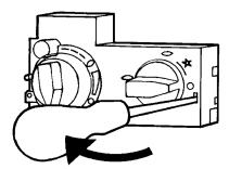
Disconnect the other end of the ignition lead from the valve body noting the route of the ignition lead.
