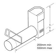
Terminal dimensions: 395 x 200 x 200 mm (H x W x D) Guard supplied Cut to length as required on site.
