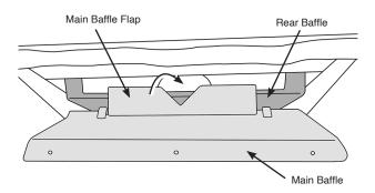
To remove the Rear baffle, undo the 2 screws.
