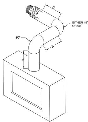
When A = 1.0 to 1.499 metres B+C = 1.0 metre max (Nat Gas - No restrictor, LPG - 75mm Restrictor)
