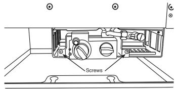
Slide the bracket slightly to the right and pull forward to access the valve connections.
