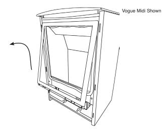
The glass frame must be refitted to the appliance following cleaning or servicing. Hold in position and secure with the screws.
