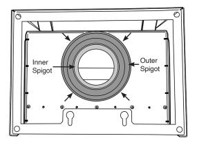
Swap the inner and outer flue spigots **only** with the inner and outer blanking plates on the rear of the appliance.
