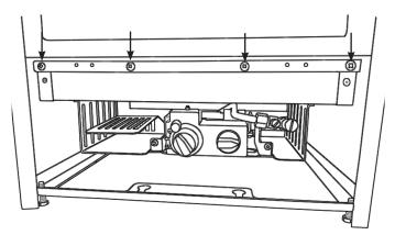
Fit the front by inserting the hooks on the back of the frame into the slots on the front of the appliance.
