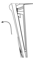
Using a screwdriver remove the 4 screws securing the window panel to the appliance.
