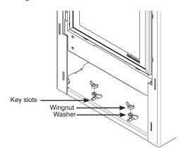
Place the 2 large washers over the studs and fix with 2 wingnuts.
