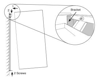
NOTE: The top rear edge of the appliance must locate between the back lip of the wall mounting bracket and the raised supports.
