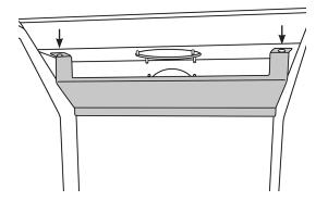
Note: When replacing the Rear Baffle ensure that the tab locates behind the rear panel slot.
