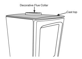
The cast top plate lifts off to give access to the inner and outer flue spigots.
