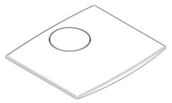
Replace the cast top. When fitted properly the cast plate should sit flush with the rear of the stove.
