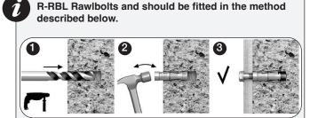
The fixings supplied for the Wall Mounted Kit are
