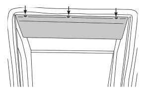
Note: when replacing the Main baffle ensure that the Main Baffle flap rests on the Rear Baffle.
