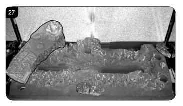
8.20 Place Log B on top of Log D. There is a hole on the underside of Log B which fits over the raised stud on Log D to secure in place. The right hand side of the log rests in the groove in the burner, see Diagram 28.
