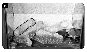
7.7 Place the pointed bottom of log D into the corner of the burner tray and rest on the location stud in log B, see Diagram 12.
