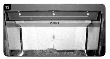
4.18 The baffle can now be removed through the front of the appliance.
