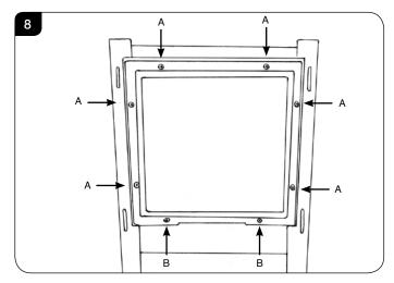
Take care to support the glass when removing the screws.
