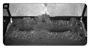
7.18 There are 3 embers. Place 2 embers in the back corners of the burner, resting in the cut outs, see Diagram 23. Place the last ember loosely at the front of the fuel bed to cover the hole in the centre.
