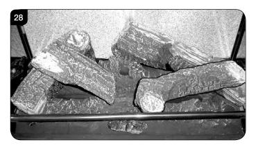
7.24 Sparingly spread an amount of the Embaglow fibres provided, covering the ports in the burner tray, Diagram 29.
