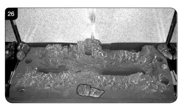
8.19 Place Log D on the left hand side of the burner. There is a hole on the underside of Log D which fits over the raised stud on the left of the burner. The back of the log should rest flat against the back panel, see Diagram 27.
