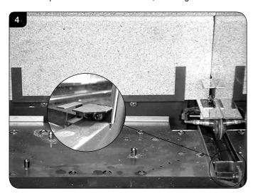
4.4 Gently lift the upper rear liner and pull forwards. With the panel raised it should be possible to remove from the liner brackets, see Diagram 5. Note: It may be necessary to use a flat object like a screwdriver to separate the two panels.
