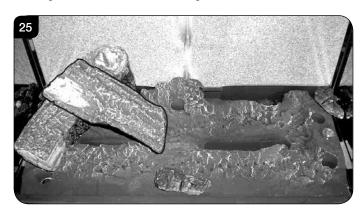
7.21 Place Log C on the right hand side of the burner. There is a hole on the underside of Log C which fits over the raised stud on the right of the burner. The back of the log should rest flush against the back panel, see Diagram 26.
