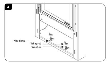
3.7 Place the two large washers over the studs and fix with two wingnuts, see Diagram 4.
