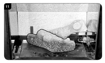
Place Log E onto the stud and behind the tag on the left hand side of the burner tray.Rest against Log B, see Diagram 12.
