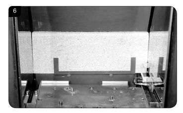
4.6 Replace all parts in reverse order ensuring the cutouts in the rear of the lower panel fit over the screws on the back of the firebox, see Diagram 7.
