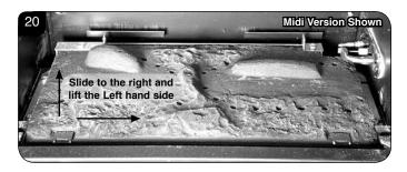
5.4 Slide the burner back to the left and out of its location. IMPORTANT: Take care when removing the burner not to damage the ceramic pad with the pilot unit attached.
