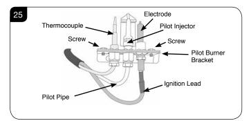
NOTE: Ensure the sealant surrounding the Electrode and Thermocouple leads is replaced if disturbed or removed whilst gaining access to these components.
