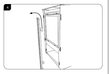
5.4 Using screwdriver remove the eight screws securing the glass frame to the appliance, see Diagram 5.Take care to support the glass when removing the screws.
