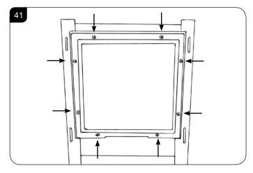
10.2 Replace ALL of the glass frame securing screws ensuring that a screw is present in all fixing slots.
