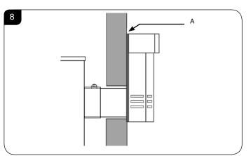
5.15 Feed the flue through the wall, making sure it runs smoothly.
