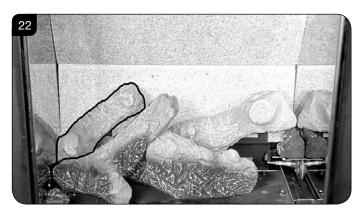
9.7 Place the pointed bottom of log D into the corner of the burner tray and rest on the location stud on log B see Diagram 23.
