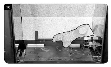
9.3 Place Log B over the two middle studs on the burner tray, see Diagram 19.
