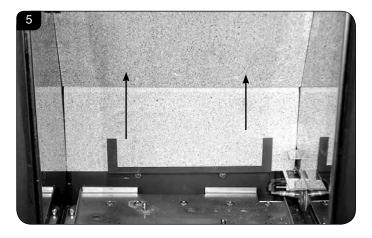
4.5 Slide the lower rear liner up and out of the lower bracket, see Diagram 6.
