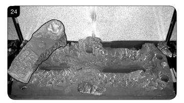
7.20 Place Log B on top of Log D. There is a hole on the underside of Log B which fits over the raised stud on Log D to secure in place. The right hand side of the log rests in the groove in the burner, see Diagram 25.
