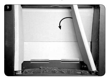
4.10 To remove the Right Hand liner first tilt inwards towards the centre of the firebox before lifting up and pulling out through the front of the firebox, see Diagram 9.
